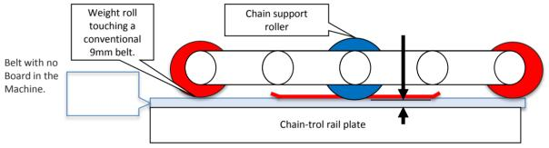
**NOTE** It is **not recommend that Spirabelt be used** on the DF-P **Shoe/Trol version**. This is the model of machine that has a series of weight rollers in the first part, the same as **Plate/Troll**, but then only Shoe bars **without intermittent weight rollers** fitted in between them. The below photo shoes **the Plate/trol version which works** perfectly with the Spirabelt providing that all the Plates are flat and adjusted correctly.
