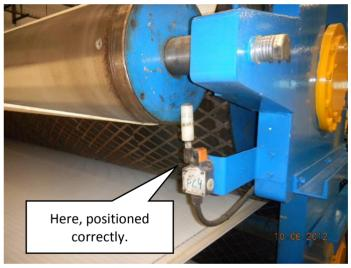
Belt should touch the paddle approximately here so that the belt edge movement does not make the belt guide mechanism over react. Air pressure to the belt guide should also be kept to a minimum e.g. 0,7 to 1,5 bar, depending on how well the mechanical parts move. Make sure that the guide mechanism is well lubricated and without air leaks.
